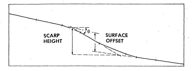
Figure 1.--Scarp profile showing definition of surface offset. Tick
