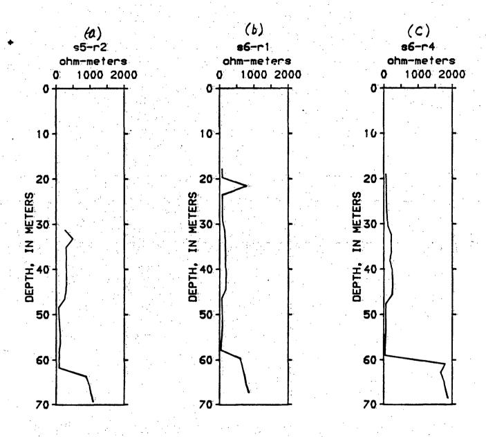
Figure 6.—Hole-to-hole measurements made parallel to the mine openings for (a) the source in hole 5, the receiver in hole 2, (b) the source in hole 6, and the receiver in hole 1, and (c) the source in hole 6, the receiver in hole 4.
