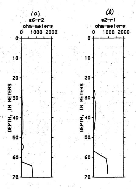
Figure 5.—Hole-to-hole measurements made across the mine openings for (a) the source in hole 6, the receiver in hole 2, and (b) the source in hole 2, the receiver in hole 1.
