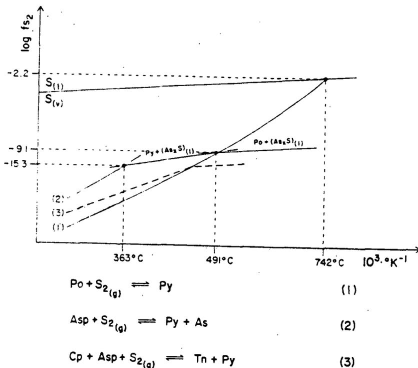
Figure 4.--Temperature (T)-sulfur fugacity ( $f_{S_2}$ ) diagram showing the possible range in T- $f_{S_2}$  suggested by equations 1-3. The thermodynamic data was taken from Clark (1960), and Barton and Skinner (1979). The Sulfur condensation curve is represented by the line  $S_{(v)}-S_{(l)}$ .
