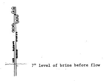
Each nut is 1" diameter, distance between nuts is 1". Mark distance down from zero feet mark (top of orange band); mark in feet and inches.
