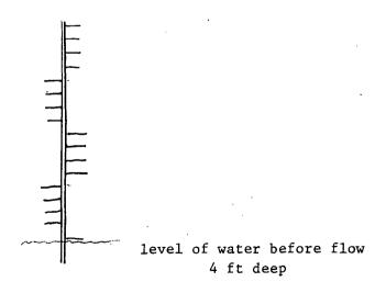
Mark water level from zero feet level down. Distance between pegs is 3". Mark level in feet and inches.
