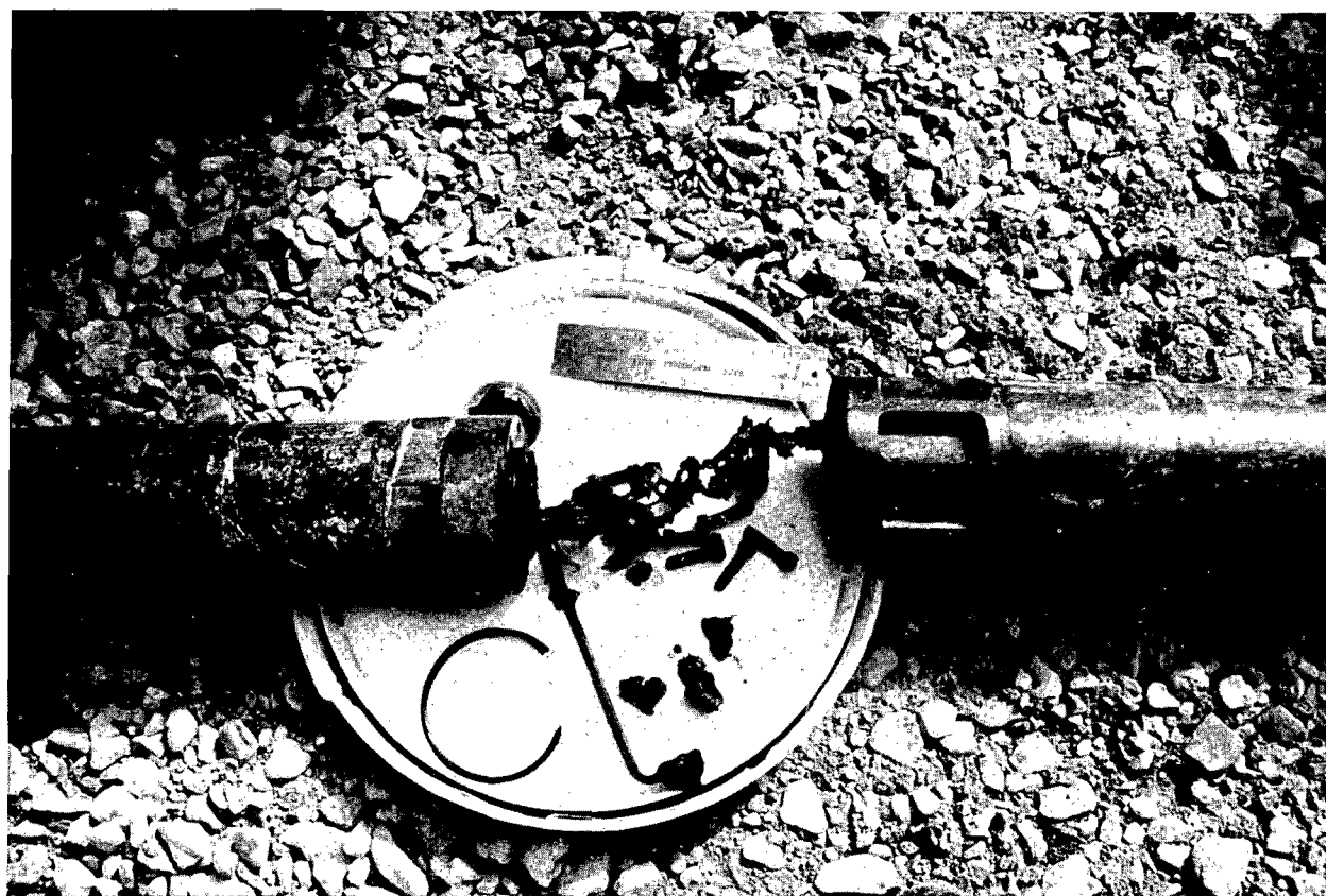
Figure 7. Photograph of "cooked" connecting wires in the bulkhead built by Sandia to connect the battery pack and sampler. The sealing design failed during runs 4 and 5 and probably during run 3. This difficulty was overcome by welding the joint together.
