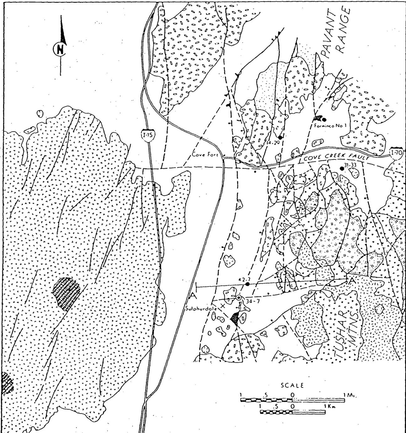
Fig. 2. Detailed geologic map of the Cove Fort-Sulphurdale area showing the location of the deep exploration wells and cross-section AA' (after Moore and Samberg, 1979; Steven and Morris, 1981).
