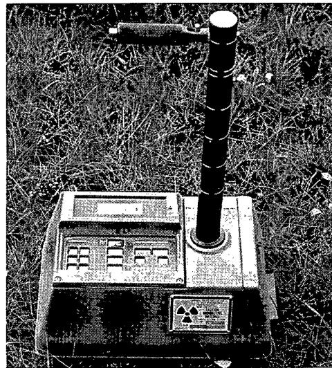
NEW calibration curves are being developed for the gauge to fit low soil densities in Southern Oregon.
