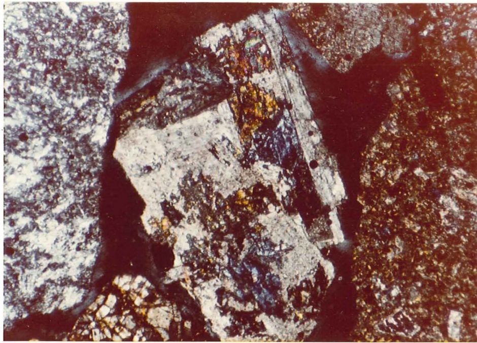
Figure 23. Epidote after plagioclase under crossed polars. (SR2A, 600 - 700 feet)
