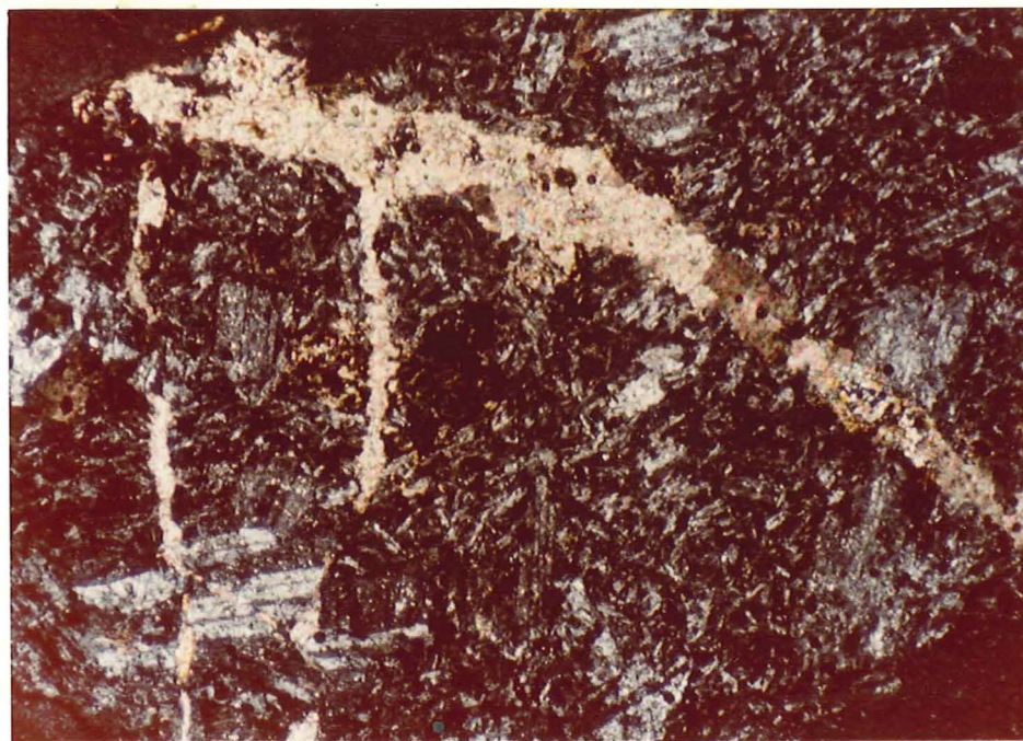
Figure 35. Calcite vein in altered volcanic rock under crossed polars. (SR2A, 500 - 600 feet)
