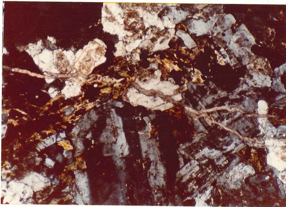
Figure 37. Calcite vein in diorite/gabbro under crossed polars. (H-1, 100 - 200 feet)
