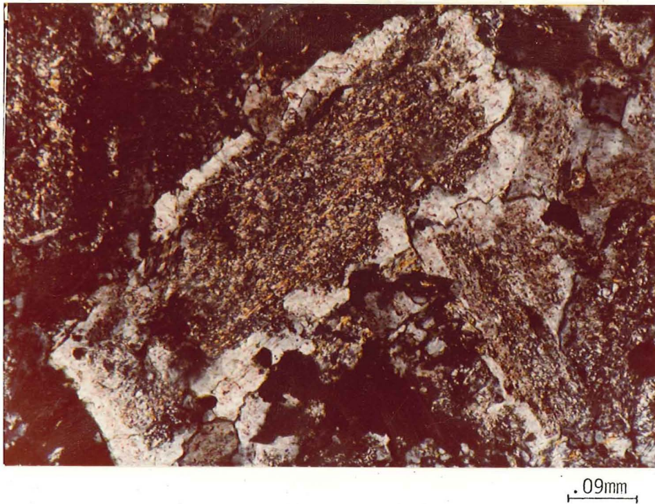
Figure 15. Sericitization of plagioclase under crossed polars. Note relatively unaltered rim. (DD-9, 1200 - 1300 feet)
