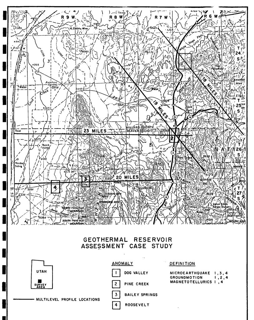
for more detail). Each ground mile of profile contains 108 magnetic measurements. The magnetic anomalies are interpreted as to meaningful geologic causes. The geology is drafted on the computerplotted and -printed profile and accompanied with a geologic report. Raw data and uninterpreted profiles will also be provided. An example of a three-level profile with description over the western rim of the Island Park Caldera is in the Appendix.
