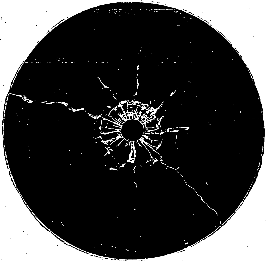
FIG. 5. Wave-generated fracture pattern in 12-in. diameter glass disc of \frac{3}{16} in. thickness after spark discharge through the centerhole.
