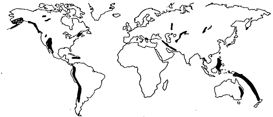
Figure 5. Most porphyry copper deposits are located either along the rim of the Pacific or in a band extending from the Middle East
