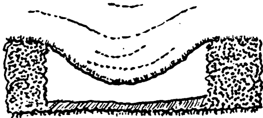
FIG. 3: Character of the Filling of the Gasified Space due to Sagging of the Roof Rocks
