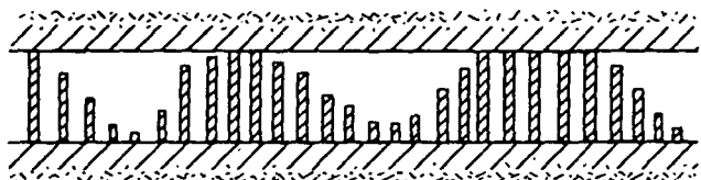
B) Mechanically and Hydraulically Equivalent Crack (schematic)
