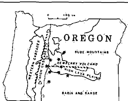
Fig. 1. Oregon, showing physiographic provinces (Baldwin, Geology of Oregon , 147 pp., 1976), major Cascade Range volcanos, including Newberry Volcano (triangles), existing USGS refraction lines (heavy-dashed lines), and planned shots (stars).
