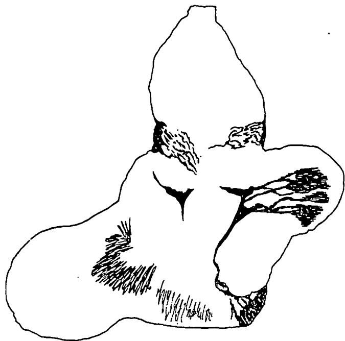
FIG. 11.—FINAL LOCATION IN THE GROUTED MASS OF FIG. 10 OF 1/6 OF THE GROUT VOLUME PLACED THIRD IN SEQUENCE
