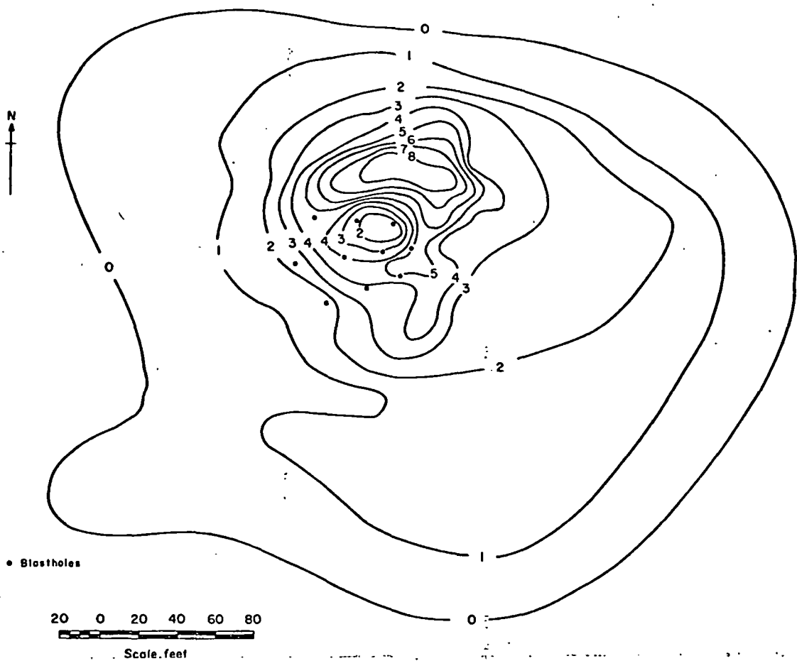
FIGURE 6. - Elevation Changes Produced by the Blast.
