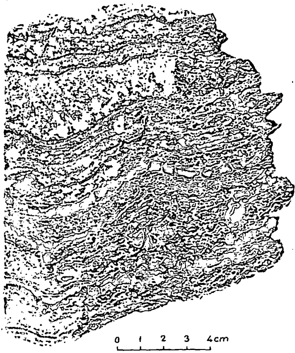
FIG. 11. Core section showing partly leached agglomerates of native sulfur; vertical contact is between sulfur-bearing and barren limestone.
