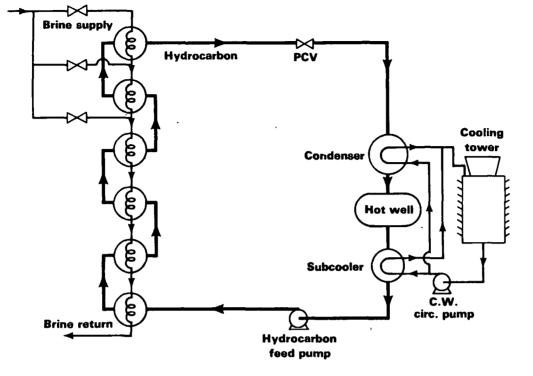
**TEST FACILITY SCHEMATIC DIAGRAM**
