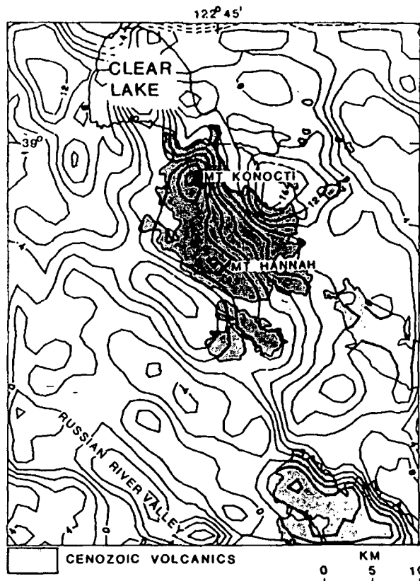
Figure 16. Residual gravity (at 2.67 \text{ g/cm}^3 ) after removal of the field from a sphere buried at 13.5 km; contour interval 2-mgal.
