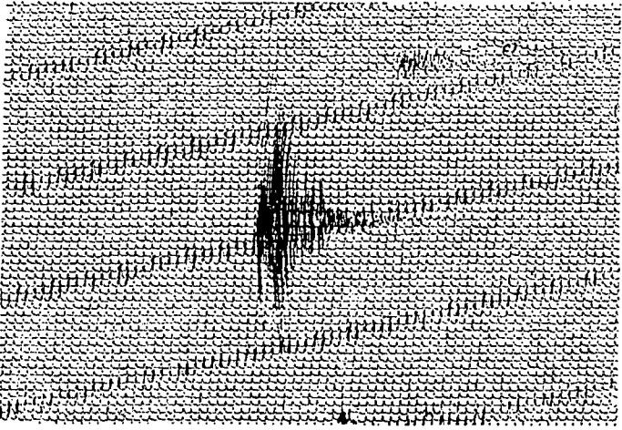
Fig. 2 - Seismogram sections from the stations RI (a) and SN (b and c). The small tick marks are second marks. Typical earthquakes with clear S-waves (a and c) and without S-waves (a and b) can be seen.
