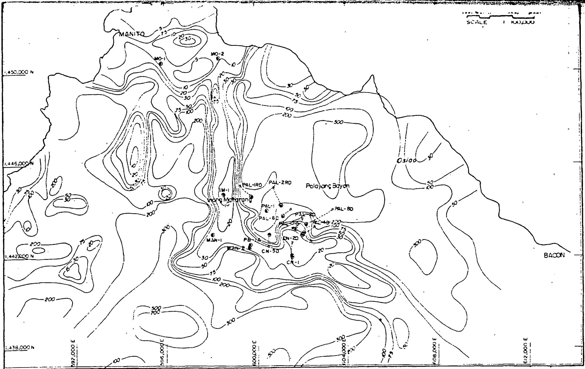
Figure 5 ISO-RESISTIVITY MAP AT AB/2 = 500 m. BACON-MANITO GEOTHERMAL PROJECT
