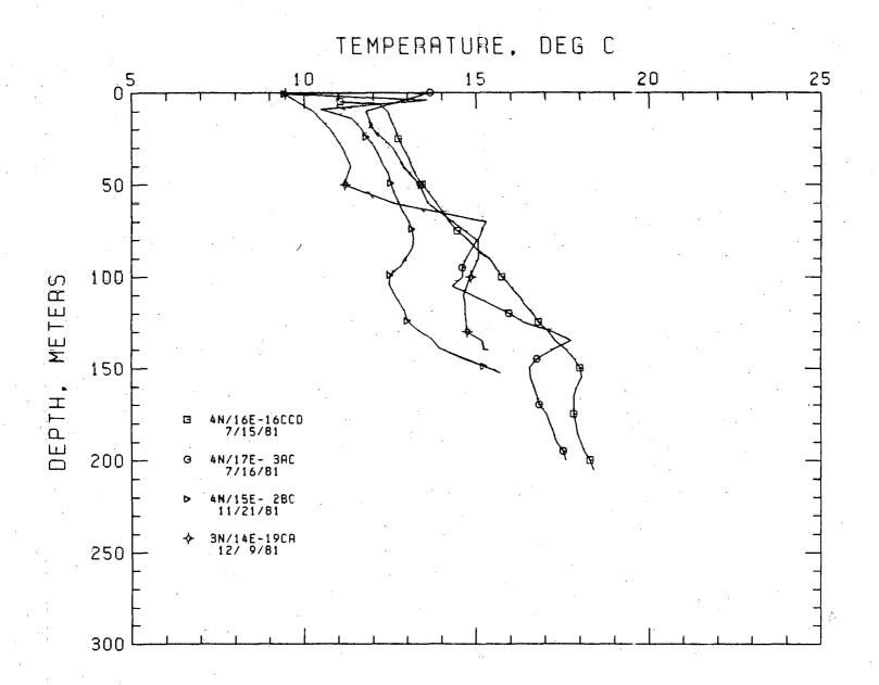
Figure 8. Temperature-depth curves for holes in the Columbia gorge. The highest gradients are in the Bonneville hot spring area, while typically low gradients are observed elsewhere. Gradients with a component of apparent lateral warm water flow are common in the area of Townships 4N/15E to 17E. Every fifth point on each log is plotted by a symbol.
