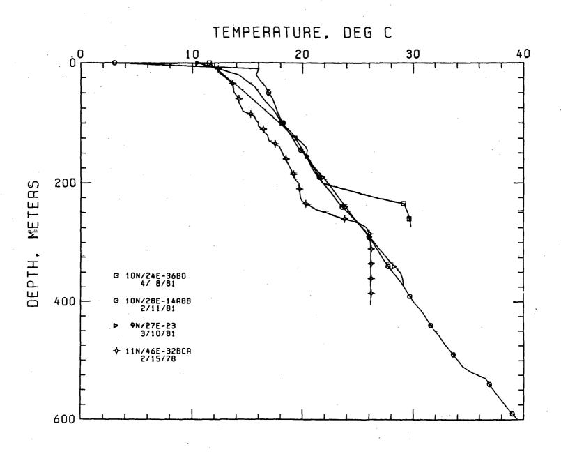
Figure 12D. Example temperature-depth curves for wells in the southern part of the Columbia Plateau. Every fifth point on each log is plotted by a symbol.
