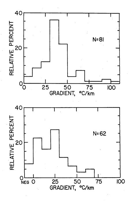
Gradients in holes logged by WRD determined this way range from over  $100^{\circ}$ C/km to less than  $10^{\circ}$ C/km. An obvious approach is to look for areas with higher-than-average gradients. Four areas that contained several holes with higher-than-average gradients were identified. These were areas referred to as the Wilson Creek anomaly (20N/30E), the Othello anomaly (16N/30E), the Yakima anomaly (13N/20E), and the Lowden anomaly (6N/33E).
