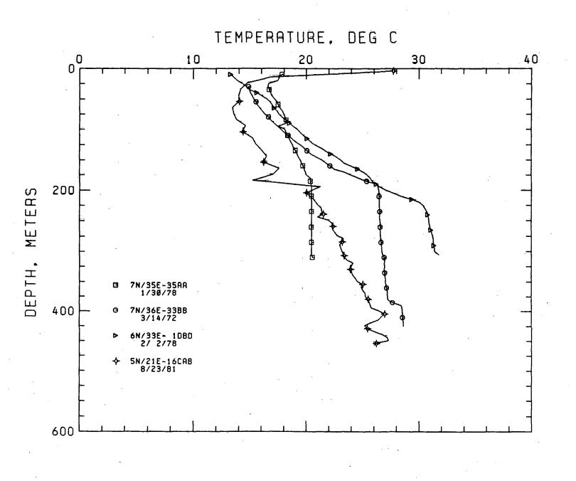
m. Hole 5N/21E-16CAB shows an irregular but linear temperature-depth curve and a relatively low gradient.
