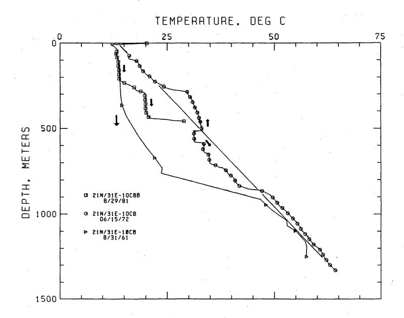
Figure 10. Temperature-depth curves for Development Associates Basalt Explorer #1. Three logs measured over a 20 year period are illustrated for this hole. Logs were obtained by R. F. Roy of Harvard University (1961), personnel from Washington State University (1972), and SMU (1981). Every fifth point on each log is plotted by a symbol.
