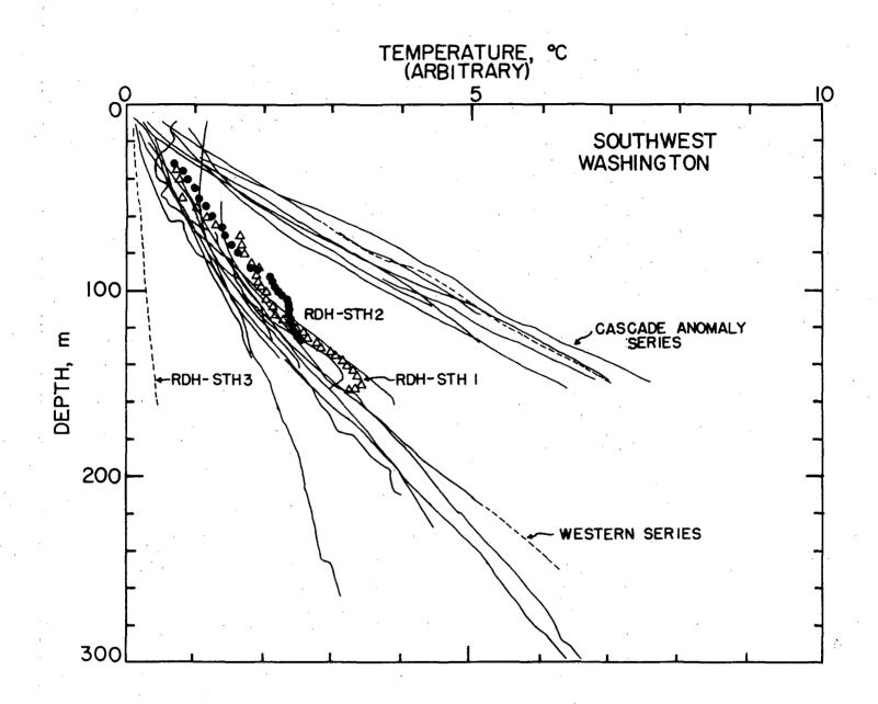
Figure 7. Temperature-depth curves for the Cascade Range and Coastal provinces. Illustrated are plots of temperature-depth data for many of the holes in the coastal provinces (low heat flow) and the Cascade Range high heat flow region (see Figure 2). Also illustrated are curves for the two holes west of Mt. St. Helens to illustrate their association with the low heat flow province.
