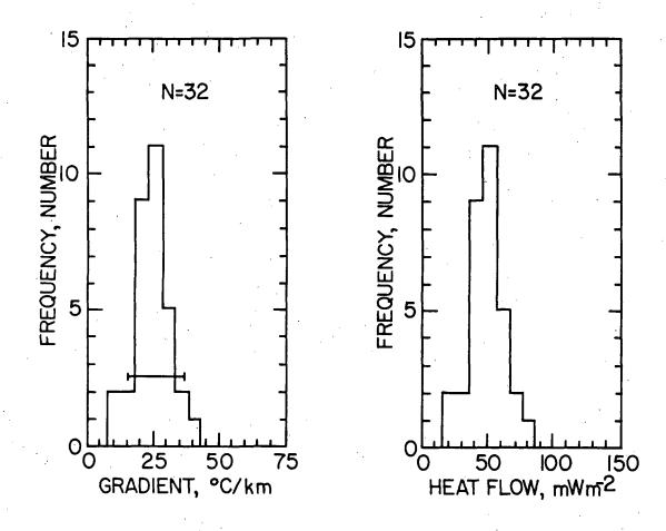
Figure 5. Histograms of geothermal gradient (A) and heat flow (B) for the coastal provinces are shown. Values are taken from Table 1. Provinces included are the Puget Lowlands, Olympic Mountains, Willapa Hills, and the Cascade Mountains west of the high heat flow zone. Band of gradients ingradient plot shows range in gradient in hole 12N/1W-9CCC associated with lithologic variations.
