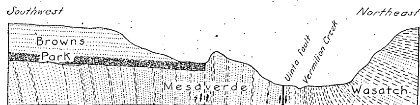
FIGURE 7.—Sketch Section showing basal Conglomerate of Browns Park Formation resting on and ending laterally against steeply dipping Mesaverde Sandstones
