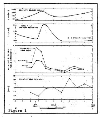
hot wells. Figure 1 contains an E-W profile of total field apparent resistivity from one of the bipole surveys which illustrates this feature. The figure also shows an approximately 4 mGal residual gravity anomaly associated with the ridge.
