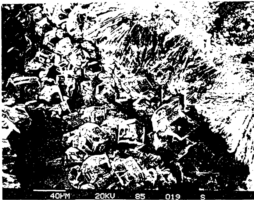
Figure 6. Scanning electron micrograph of a partly dissolved phillipsite filling between breccia fragments at 812-m depth.
