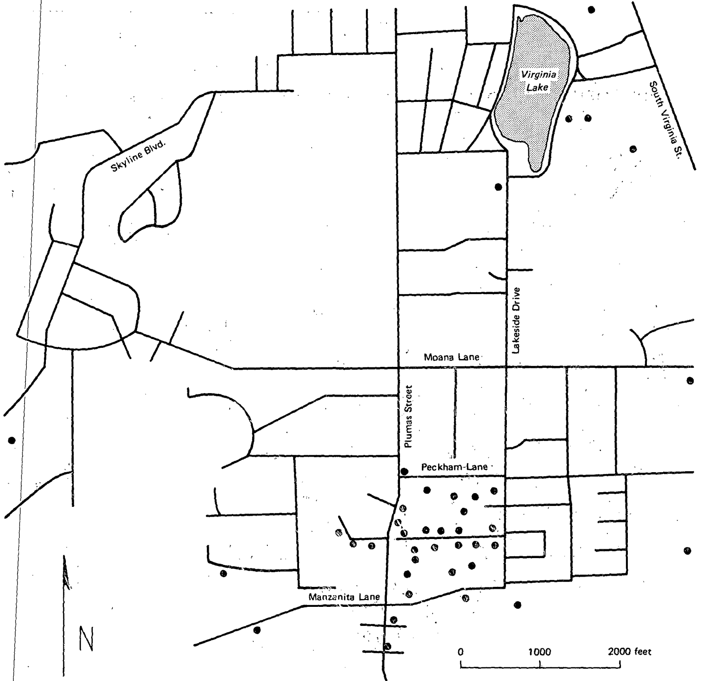
Map showing locations of shallow thermal wells in southwest Reno that are used for space heating, domestic hot water, and swimming pools (from unpublished map by R. B. Scheibach, 1974).
