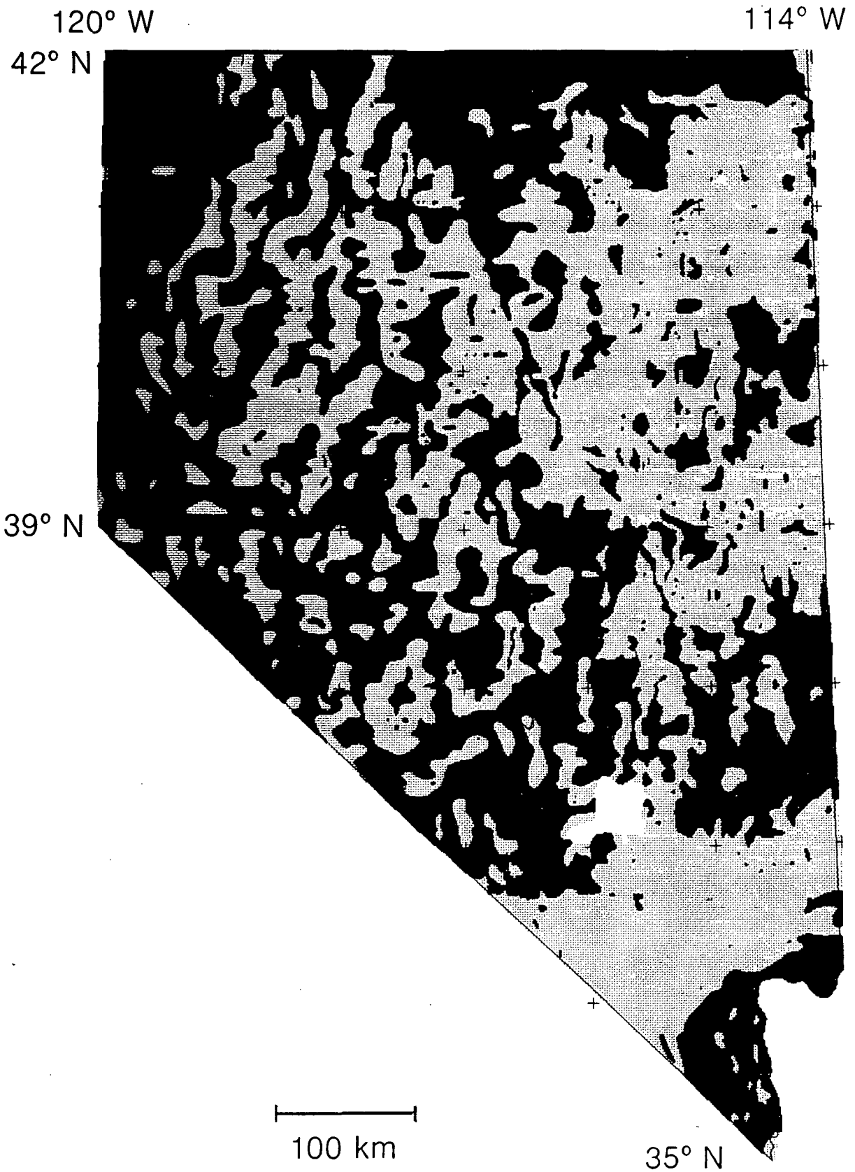
Fig. 5. Location of shallow magnetic sources in Nevada as interpreted from NURE magnetic profiles. Areas with magnetic sources within 1 km of the topographic surface are shown in black; areas without magnetic sources within 1 km of the surface are shown in stipple pattern. Blank area indicates insufficient data to make a reliable interpretation.
