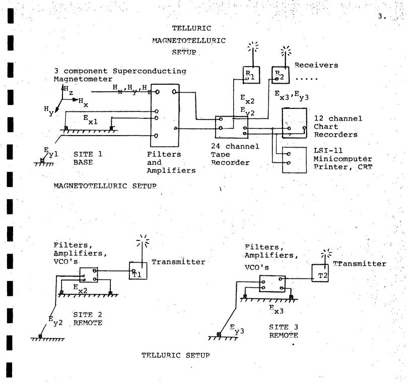
Figure 1. Magnetotelluric-Telluric Instruments
