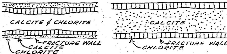
Minor fractures display either a calcite and chlorite, or a calcite and a black mineral(?) mineralogy. Vesicles are present and are filled with calcite and/or calcite rimmed with chlorite. The core shows moderate hydrothermal alteration.
