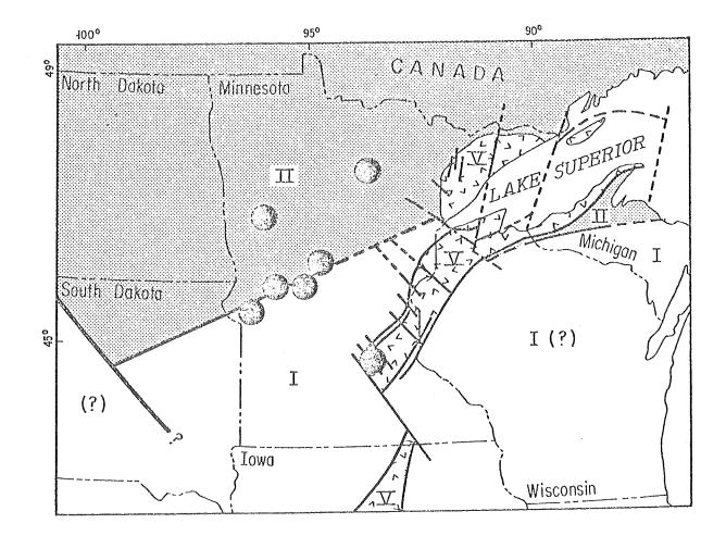
Figure 1. The fundamental Precambrian basement terranes of Minnesota and adjacent areas as they would appear if overlying sedimentary strata were removed. Black circles are the locations of historic earthquakes within Minnesota. The map does not show the lower Proterozoic rocks of terrane III (Animikie basin), terrane IV (Sioux Quartzite) or rocks of Phanerozoic age.
