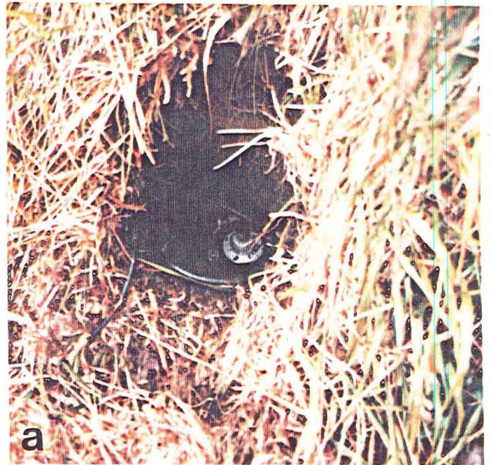
Figure 16. Microearthquake recording station: a) Vertical-component seismometer; b) Checking timing on a MEQ-800 smoked paper drum recorder; c) Resulting record for one day, containing a regional earthquake.
