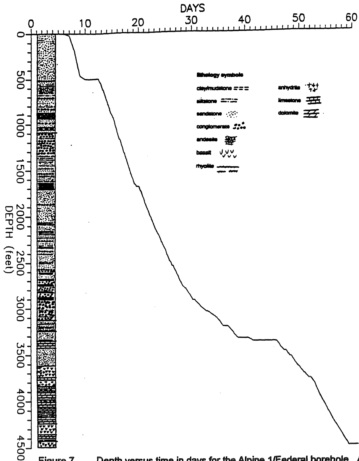
Figure 7. Depth versus time in days for the Alpine 1/Federal borehole. A summary stratigraphic column is shown for comparing geology with daily drilling progress.
