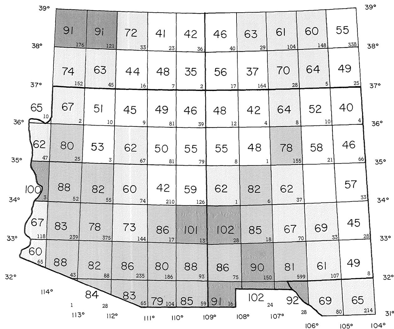
**Figure 12.** Silica geotemperatures averaged over a  $1^{\circ} \times 1^{\circ}$  grid and the major tectonic provinces of the southwest.
