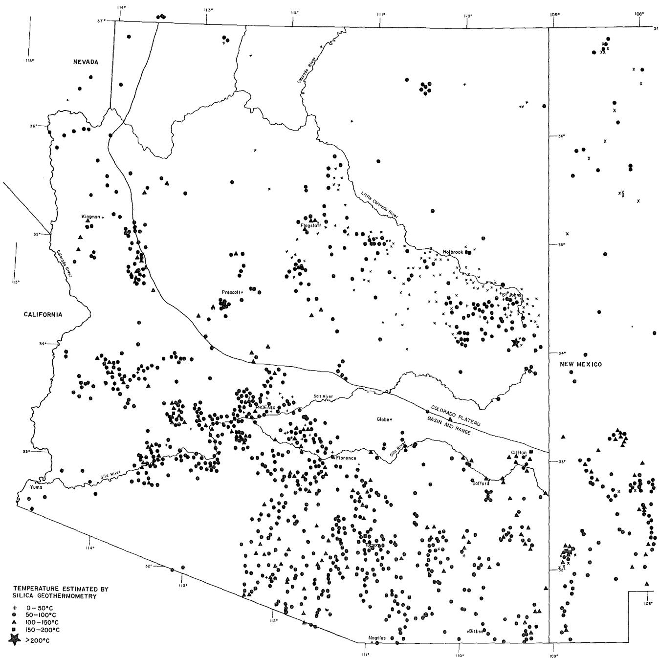
Figure 3. Na-K-Ca geotemperatures for waters from Arizona, western New Mexico, and southwestern Utah. Calculations based on data from Table 2 and from the U.S.G.S. water quality file.
