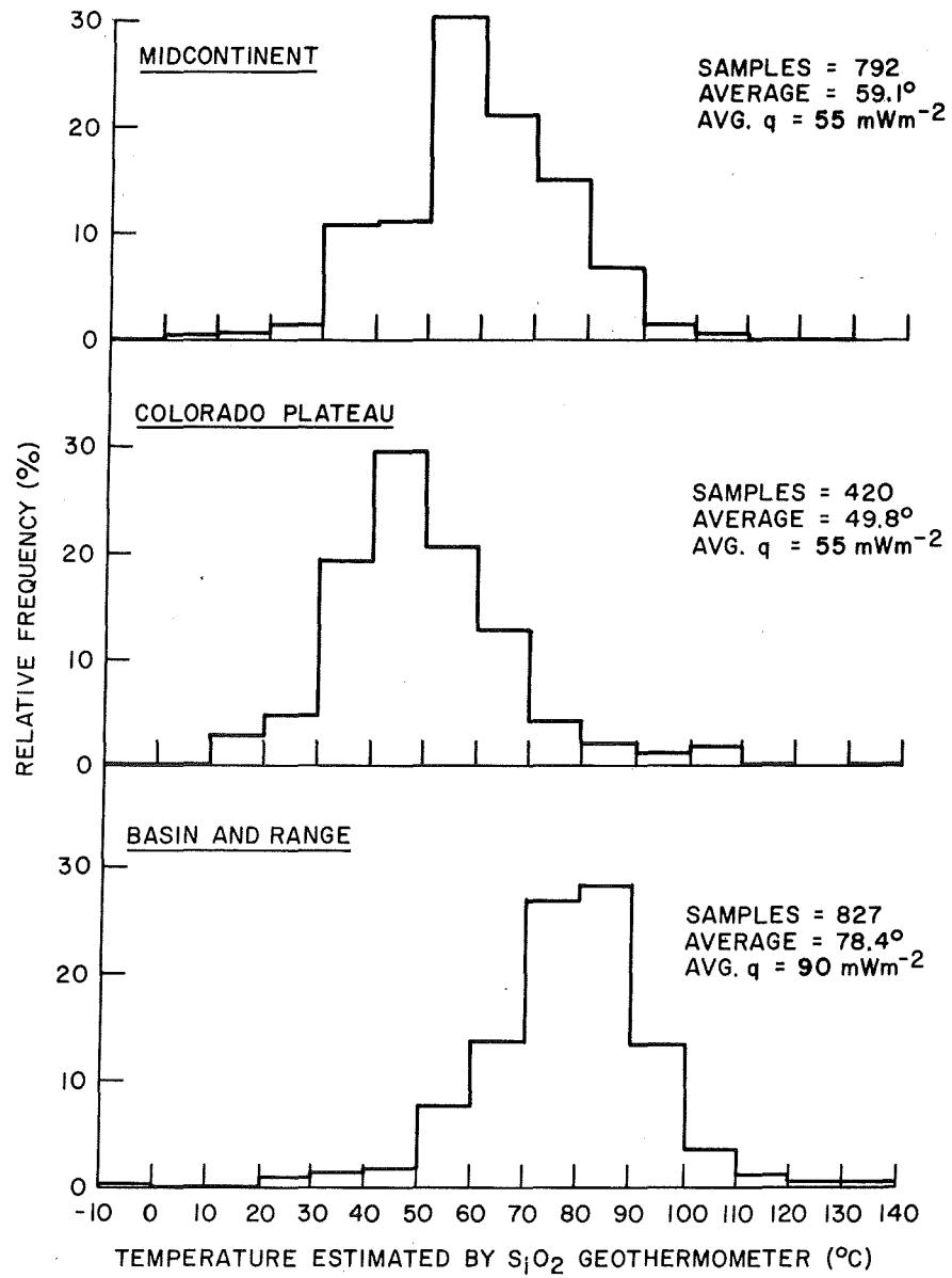
Figure 11. Silica geotemperatures averaged over a  $1^{\circ} \times 1^{\circ}$  grid.
