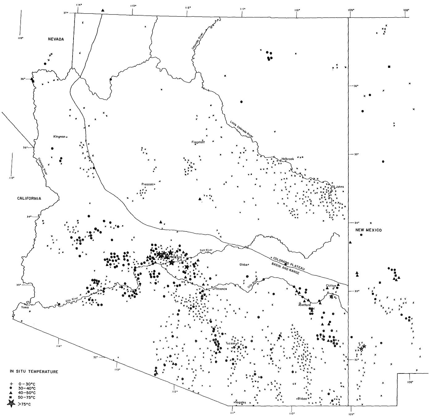
Figure 2. Silica geotemperatures for waters from Arizona, western New Mexico, and southwestern Utah. Calculations based on data from Table 3 and from the U.S.G.S. water quality file.
