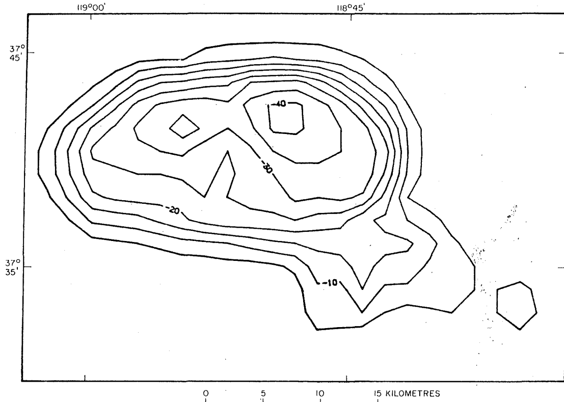
Fig. 2. Residual Bouguer gravity map of Long Valley area. Contour interval is 5 mGal.
