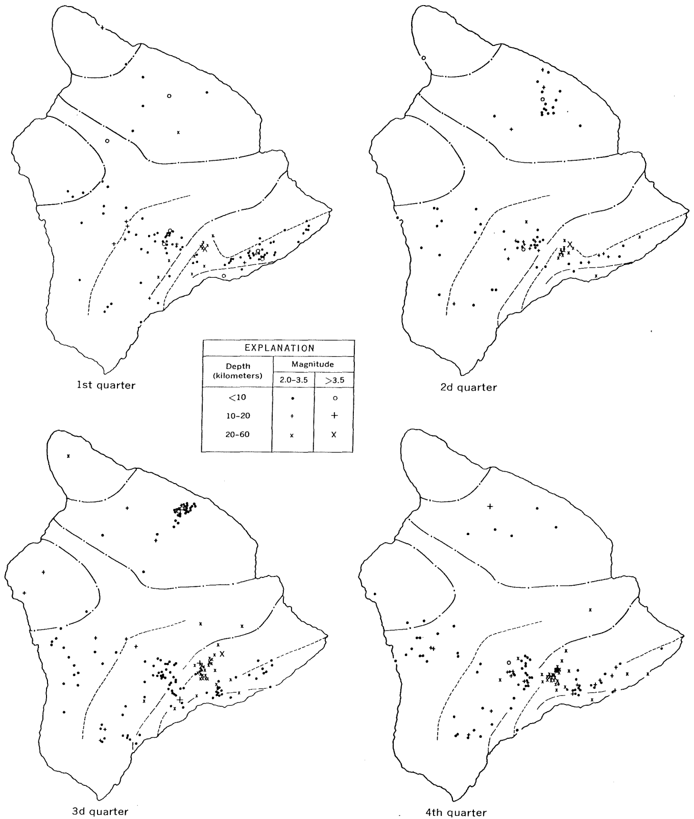
FIGURE 2.—Plot of epicenters of earthquakes having a magnitude of 2.0 or greater beneath the island of Hawaii during each quarter of 1967. Dot-and-dash lines are boundaries of volcanic systems, long-dashed lines are fault systems, and short-dashed lines are rift zones. Geographic names are shown in figure 1.
