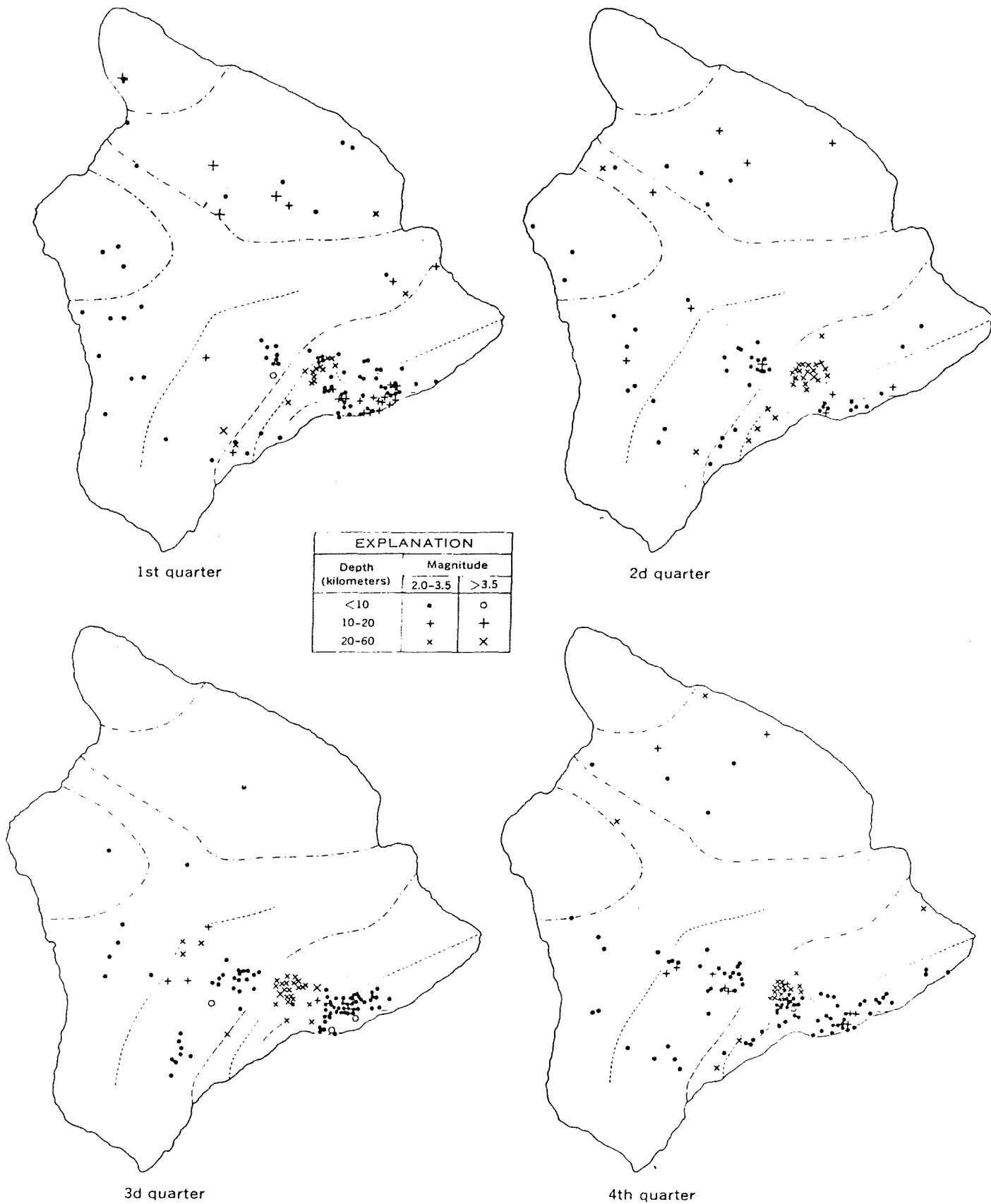
Figure 7. Quarterly plot of epicenters of earthquakes of magnitude 2.0 or greater beneath the island of Hawaii during 1965. Dot-and-dash lines are boundaries of volcanic systems, long-dashed lines are fault systems, and short-dashed lines are rift zones. Geographic names are shown in figure 1. (from Koyanagi, 1968)
