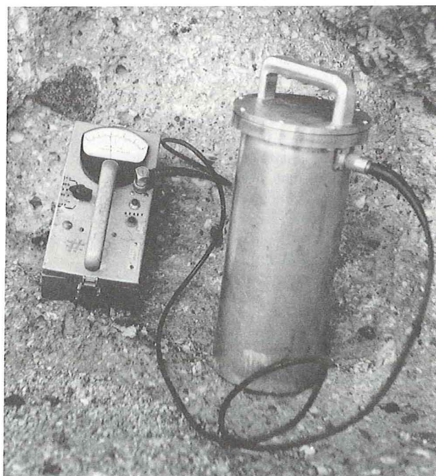
Figure 2. Field gamma counter. The 3-in. by 3-in. NaI(Tl) scintillation crystal and photomultiplier tube are encased by the steel cylinder, and are connected to the accompanying count-rate meter.
