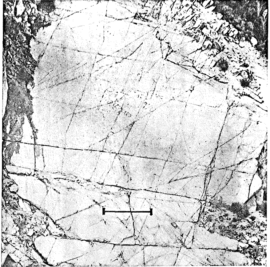
Outcrop of the porphyritic Schultze Granite demonstrating the geometry and distribution of flow and diffusion porosity. Continuous fractures, which cross cut outcrop, represent flow channels, and discontinuous fractures represent diffusion porosity. Scale bar is 5 m.
