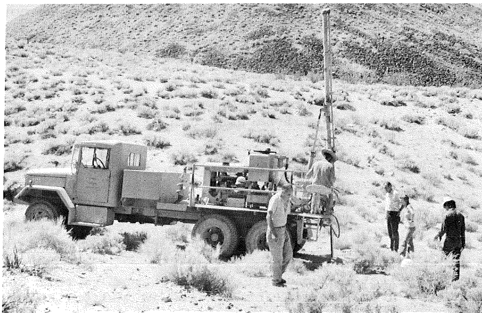
FIGURE 2: A truck-mounted hydraulic posthole-digger was used at Coso.
