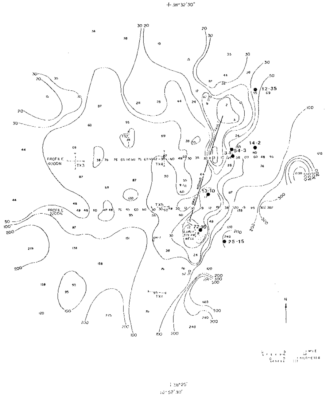
FIG. 10. CSAMT apparent resistivity map of Roosevelt Hot Springs KGRA. Frequency = 977 Hz. Areas less than 10 \Omega -m are shaded.
