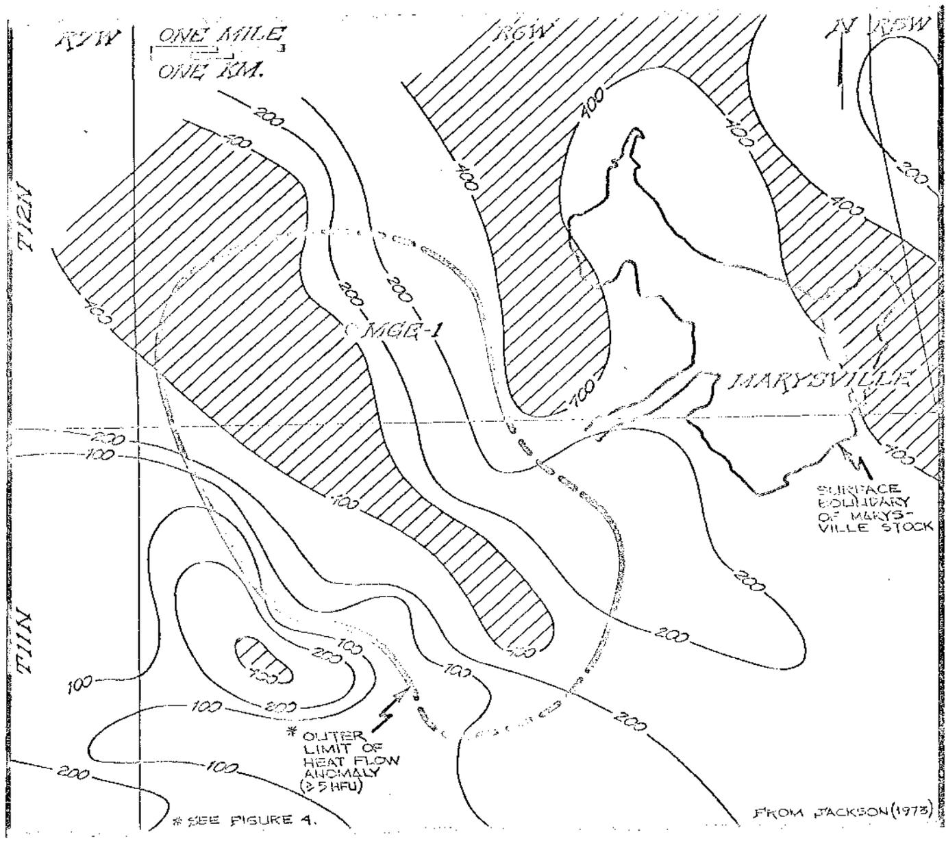
FIGURE 7. SHALLOW APPARENT RESISTIVITY MAP OF THE MARYSVILLE GEOTHERMAL AREA BASED ON ROVING DIPOLE RESISTIVITY SURVEY. VALUES ARE IN OHM-METERS
