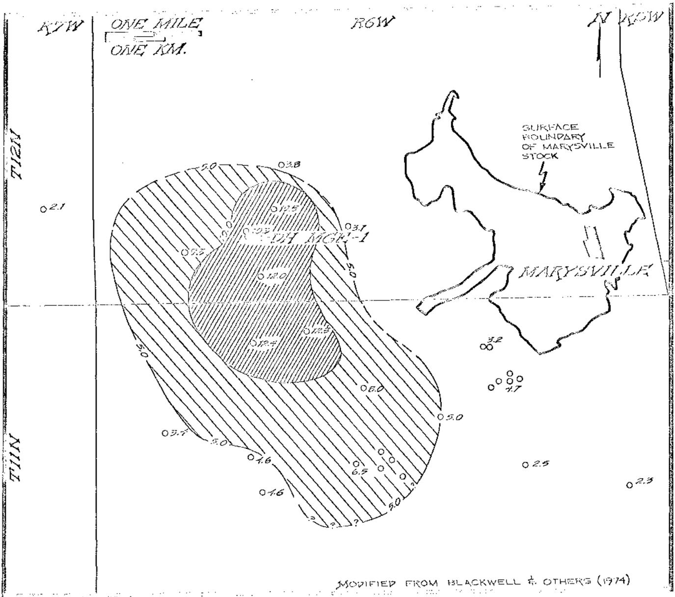
FIGURE 4. SHALLOW HEAT FLOW MAP OF THE MARYSVILLE GEOTHERMAL AREA. VALUES RECORDED ARE HEAT FLOW UNITS (HFU =  $\mu\text{cal}/\text{cm}^2\text{sec}$ )
