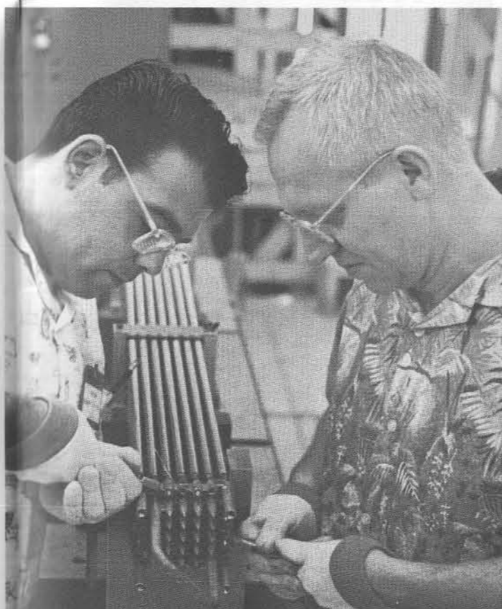
Uranium fuel is made in pellet form, sealed in long tubes and bundled. These technicians at a General Electric Company nuclear facility are assembling a loaded fuel bundle. Humboldt Bay's nuclear unit has 172 of these fuel assemblies.
