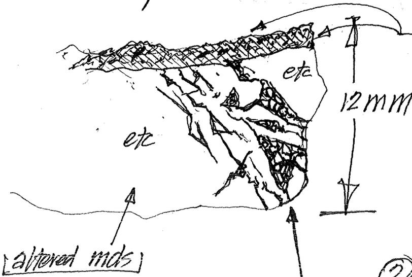
③ tectonic crush microbreccia, clasts < 0.1mm - 0.7mm subequant, commonly granulated edges, loosely cemented with fxlh - vxlh, specular hematite and lesser ultra-fxlh quartz
