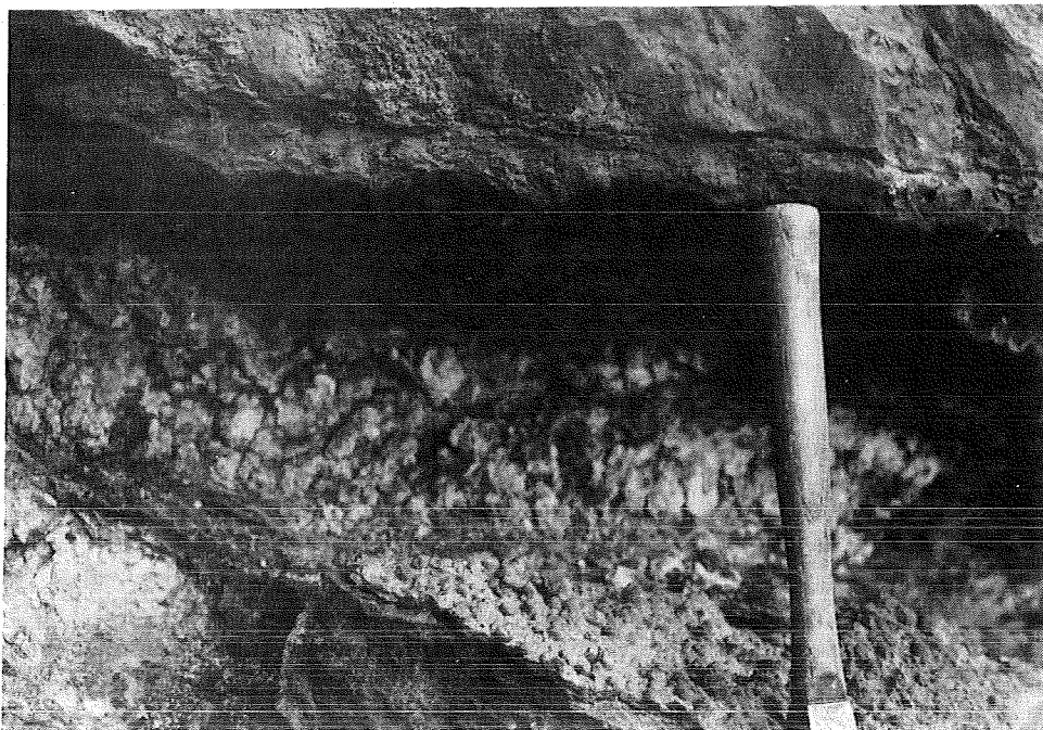
FIGURE 3. View of the largest vein present at the West End mine shown in Figure 1. The vein is about 40 cm in width and consist of 2-4 cm of clear to petroliferous quartz deposited on each wall of the vein and a central zone of hydrothermal clay.
