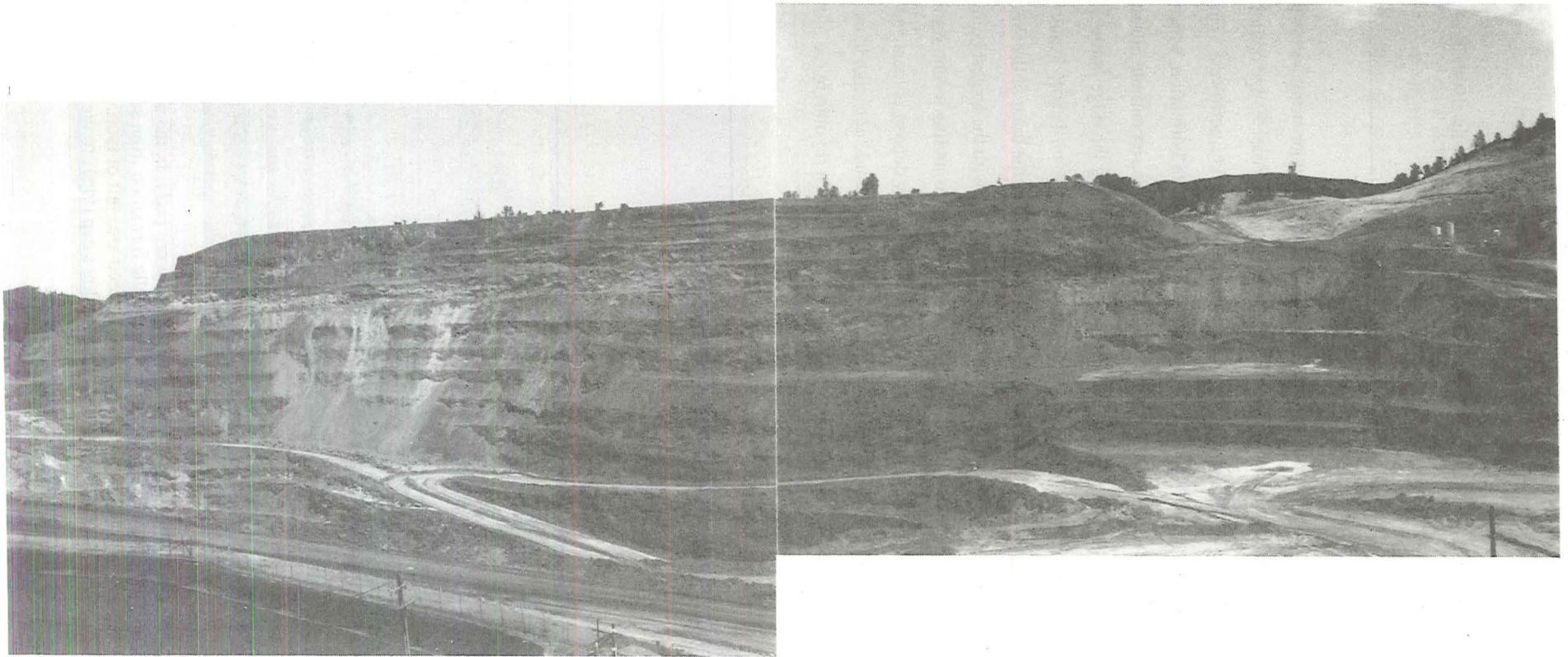
FIGURE 5. Overview of the northeast wall of the south ore body at the McLaughlin gold deposit. On the skyline, Gail Ridge is capped by a basaltic andesite flow about 20m thick (see Figure 6). The flow caps the hill to the extreme right (east) and was deposited on adularized mudstones and shales of the Knoxville Formation. The Johntown neck, a basaltic-andesite plug with an agglomerate apron, occurs in the right foreground. Agglomerate beds in the Gail maar deposits to the left (west) of the Johntown neck hosted mercury mineralization (see Figure 6). The San Quentin sinter occupied the area in the central part of the open pit, see Figure 6 for comparison to view prior to development of McLaughlin gold deposit.
