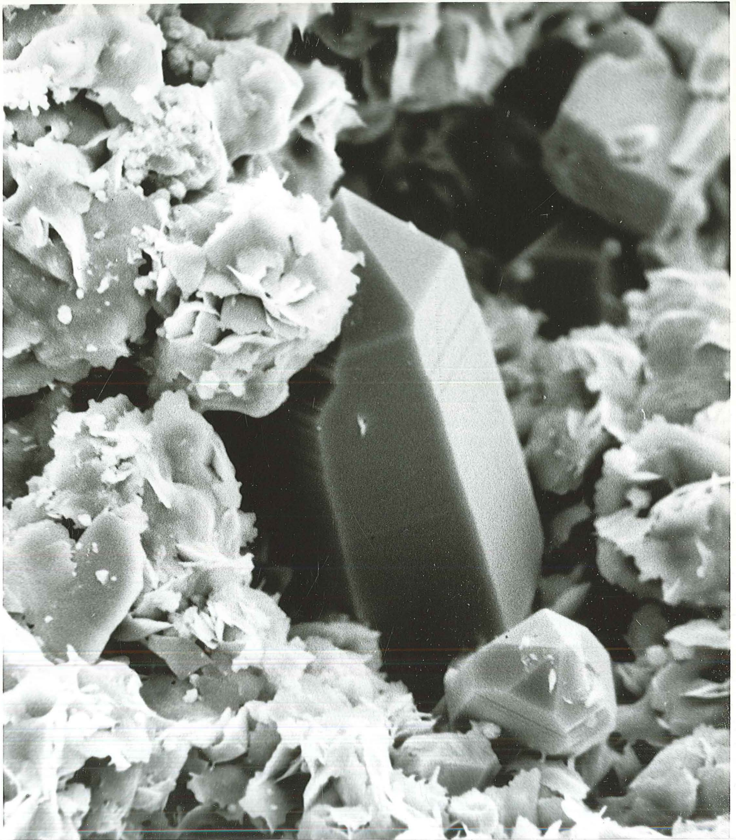
SEM photomicrograph of hydrothermal quartz and illite lining a vug in quartz-sericitized rhyolite ash-flow tuff; core from 42.2m depth in corehole VC-2A, Valles caldera, New Mexico. Largest quartz crystal shown is 0.3 m in diameter. Photo by Tom Little
