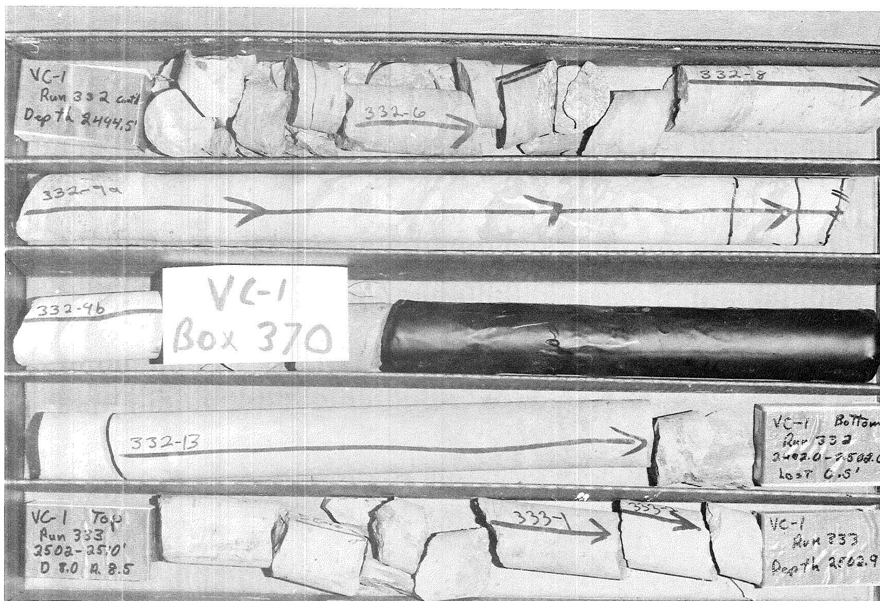
Fig. 20. Core runs 332 and 333 from the Madera limestone. Note recovery in very fractured zone, depth interval 2494.5 to 2502.6 ft (Box 370).
