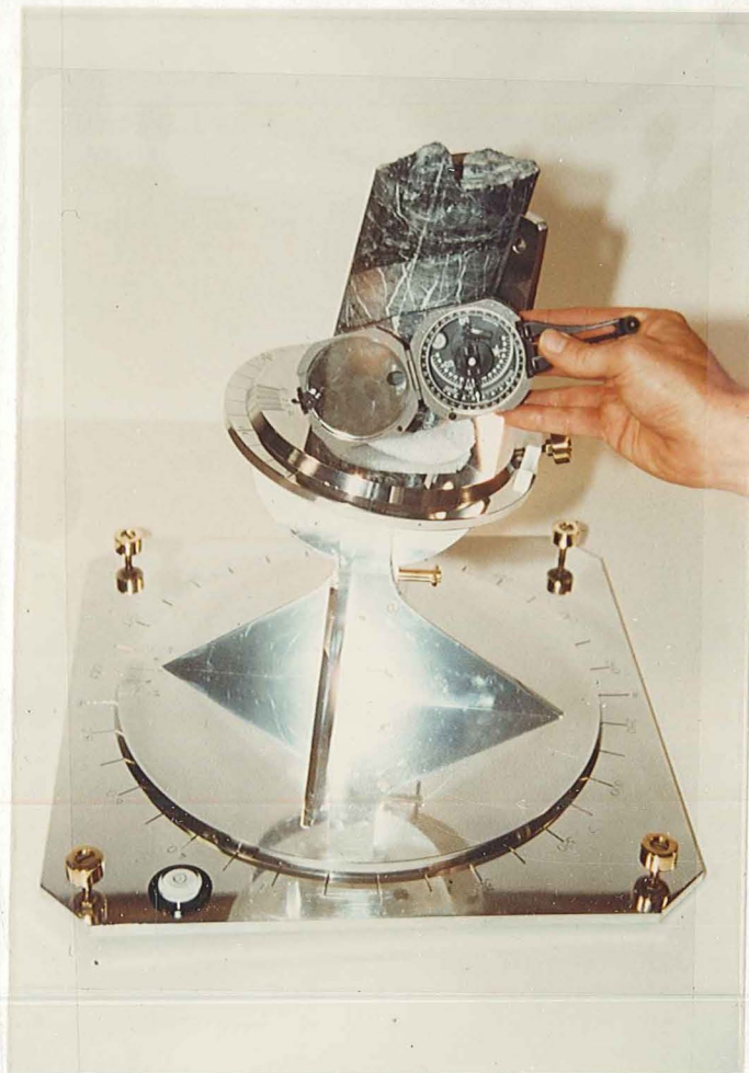
PLATE 2 GONIOMETER FOR RE-ORIENTING 4" CORE FROM PRATI 5
