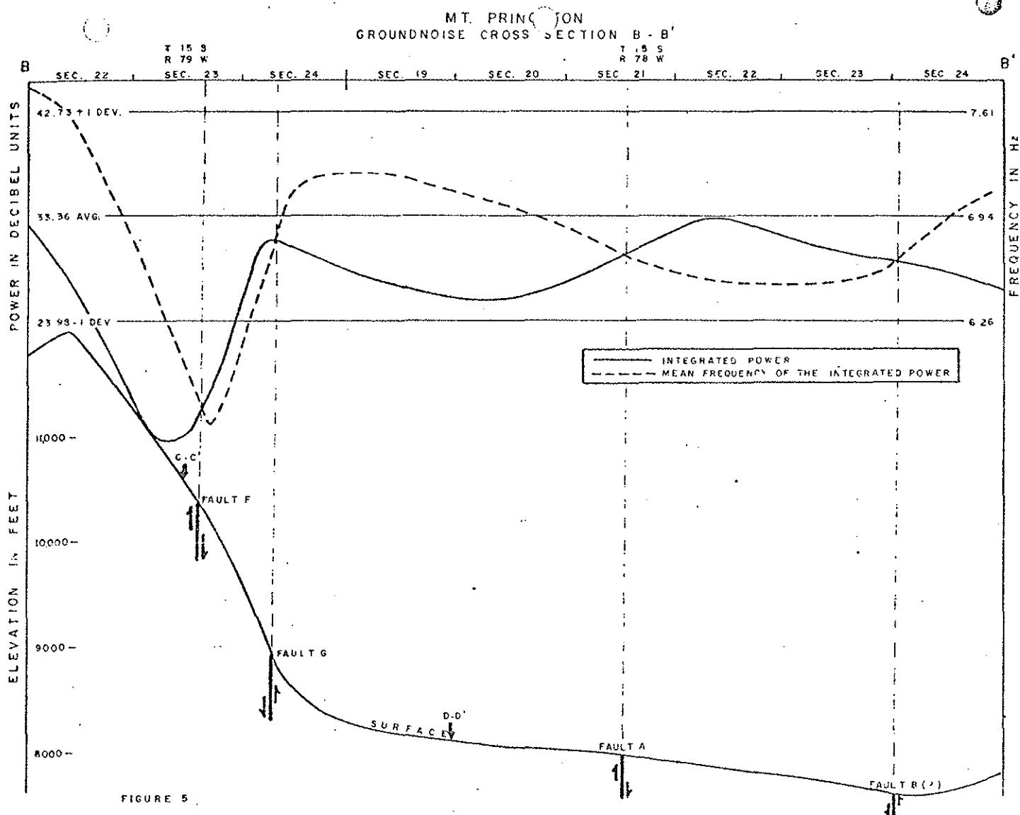
Figure 6A. Locating of faults by intersections of integrated power and mean frequency profiles, according to Senturion Sciences.
