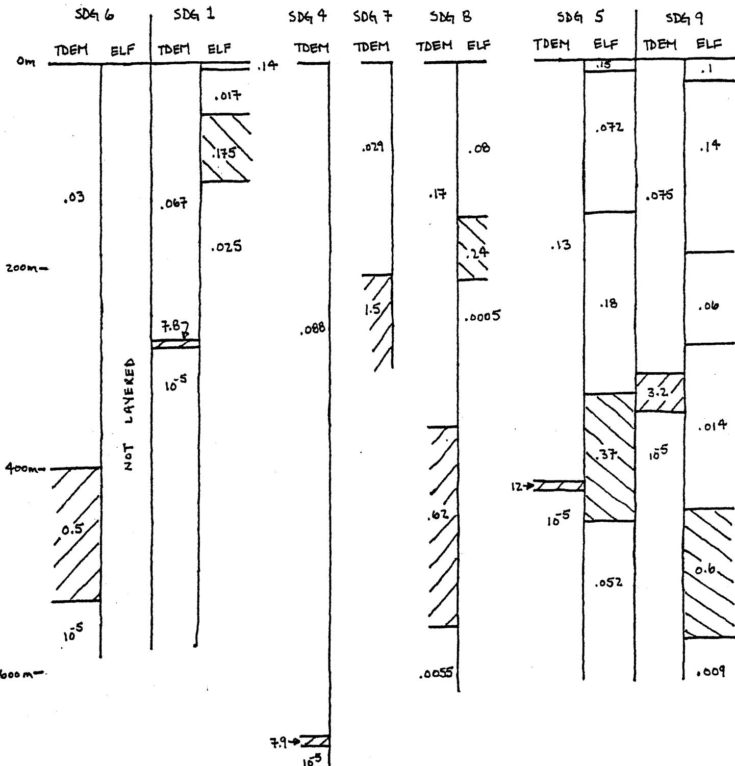
Figure 2. Cross-section perpendicular to the wire source in Figure 1 showing both TDEM and ELF sounding interpretation. Horizontal distances are not to scale.
