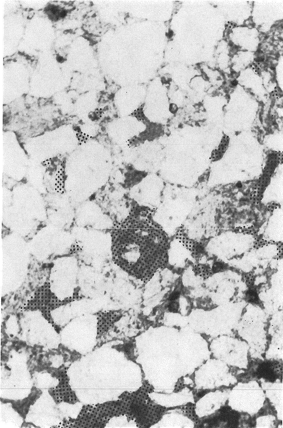
Figure 29. Photomicrograph of sandstone at 915.3 m depth in well M-20 showing porosity in dot pattern. On the right side of the view an area cemented by carbonate is present. The packing arrangement of detrital grains is similar in both cemented and cement-free areas. View is 1.2 mm across.
