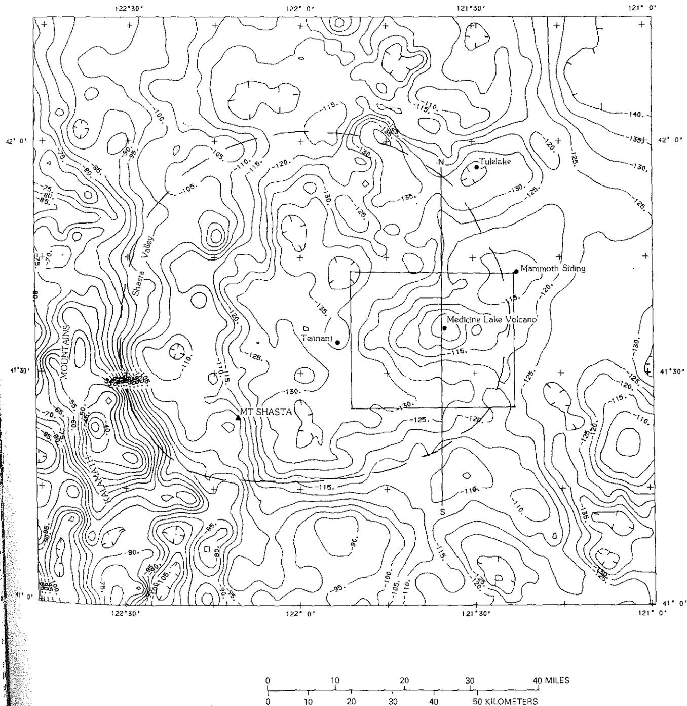
Figure 3. Complete Bouguer gravity map of area near Medicine Lake and Mt. Shasta, California, reduced at density of 2.2 g/cm<sup>3</sup>, and contoured at 5-mgal interval. Hachures indicate gravity lows. Dashed circle outlines shape described by LaFehr (1965) and Heiken (1976). North-south line indicates profile in Figure 2; rectangle is area shown in Figure 4.
